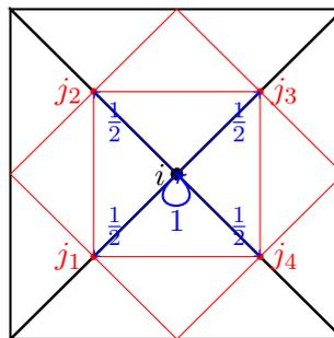
Assume the large black triangles were (red) refined and the red triangles are the result. Then the prolongation operator  $T^{l \rightarrow l+1}$  distributes the value of the basis function in the node  $i$  on level  $l$  to the basis functions in the node  $i$  on level  $l + 1$  (with the weight 1) and to the (new) basis functions in the nodes  $j_1, \dots, j_4$  (with the weights  $\frac{1}{2}$ ).
