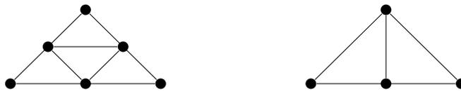
Figure 1: Left: red-refinement. Right: green-refinement.
