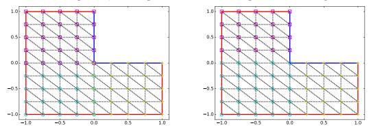
e) For both cases, compute the local problem (sub)matrices  $K_{\lambda} = r_{\lambda}Kp_{\lambda}$  of the global stiffness matrix K computed from programming exercise 3. *Hint*: This can be done using only **array** slices.
