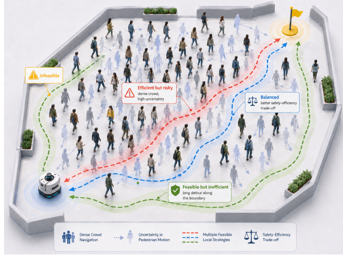
Figure 4.1: Schematic illustration of robot crowd navigation. The robot moves toward its goal while accounting for nearby pedestrians and their possible motion. The candidate routes illustrate the trade-off between navigation efficiency and safety: a shorter route may pass through a more crowded region, whereas a longer detour may provide greater clearance. The illustration was generated with ChatGPT and is included only to provide visual intuition.
