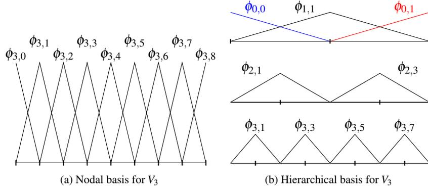
**Fig. 1:** Nodal and hierarchical basis of level  $n = 3$ .
